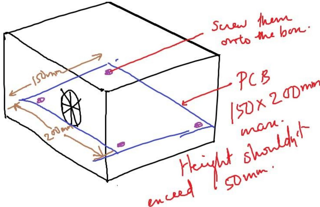
Design objective here is to make a cabinet (enclosure) for the printed circuit board.
