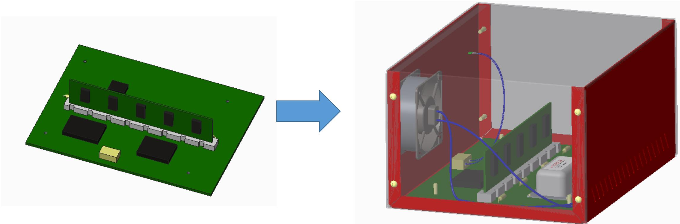
Shows the Top-Down approach in designing a cabinet from the inputs given.
